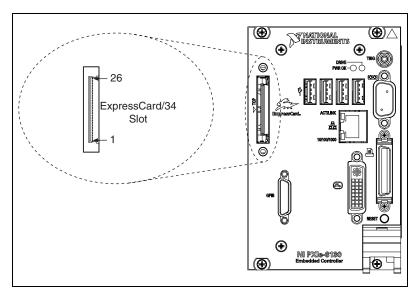
Figure 3-9. ExpressCard/34 Slot Location and Pinout
